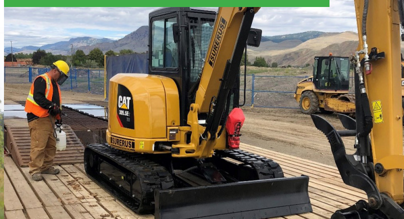
Application of dilute bleach solution for disinfection
