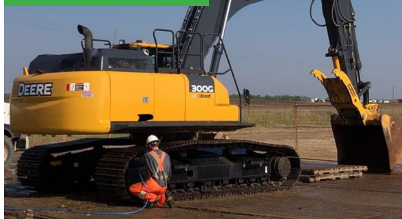
Application of dilute bleach solution for disinfection
