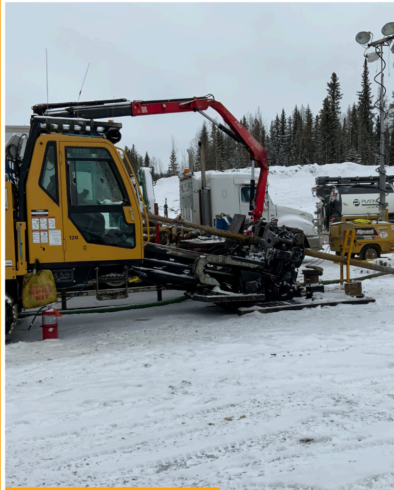
Horizontal Directional Bore (HDB)
